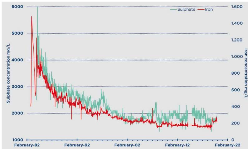
**Fig. 4:** Example of a ‘first flush’: development of the measured iron and sulphate concentration in the discharge from the Ibbenbüren western district via the Dickenberg drift
