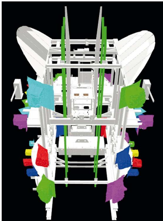
**Fig. 2:** 3D model of the shaft inset frame on level 5 showing the position of the holings
