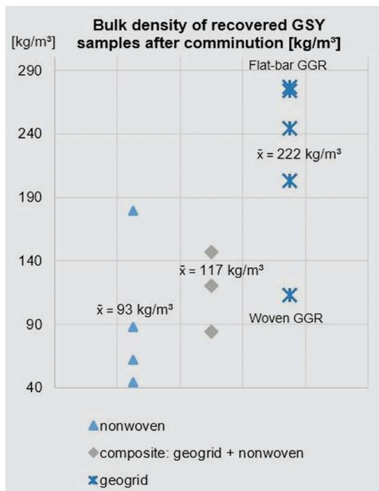
**Fig. 7:** Bulk densities of recovered GSY samples after comminution [kg/m³]
