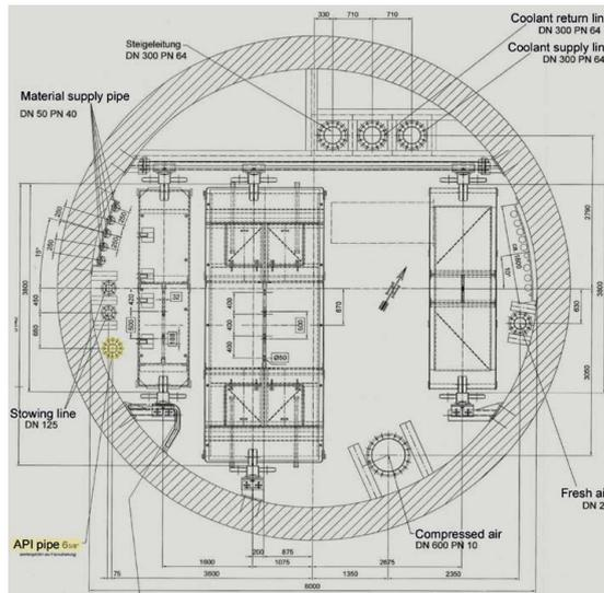
**Fig. 9: Shaft cross-section with API slick line**
