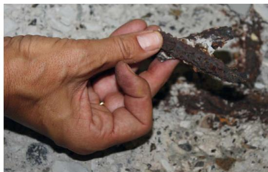
Fig. 5: Reinforcement corrosion in a non self-healing water-bearing separating crack in a WU structure
