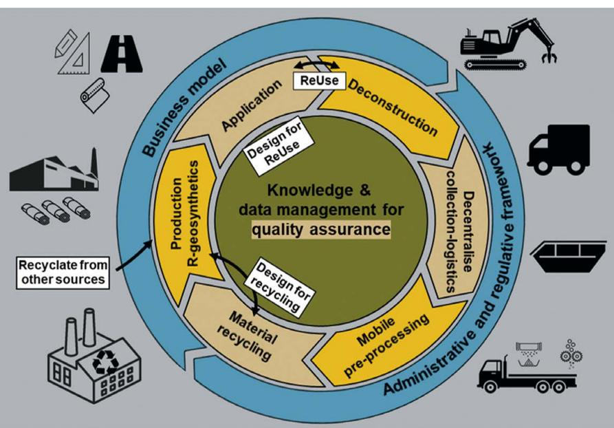
**Fig. 11:** Concept for closing the loop for geosynthetics
