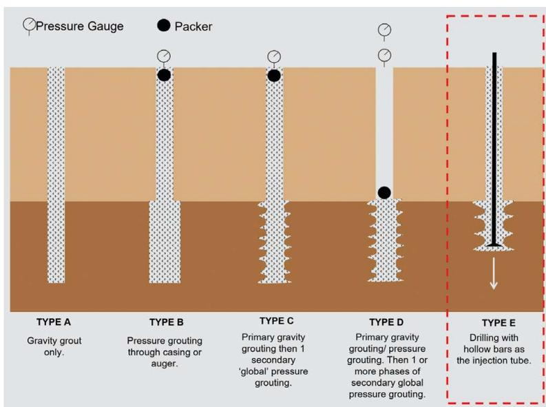
**Fig. 2:** Micropile classification recognized in the United States [1]
