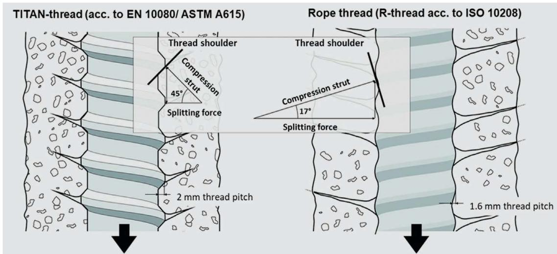
**Fig. 3:** Cracking pattern observed under tensile loading for Titan thread (left) and Rope thread (right) [12]
