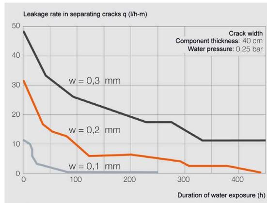
Fig. 4: Typical leakage rate for separating cracks under water exposure and with self healing
