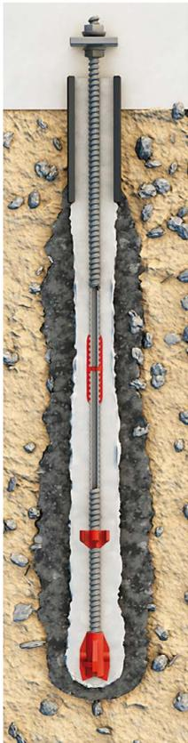
**Fig. 1:** Cross-section through typical Type E micropile
