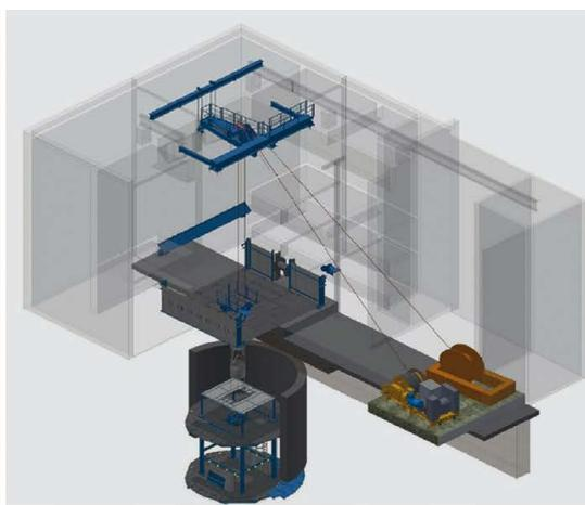
**Fig. 14: Hoist and scaffold installation that has to be assembled and dismantled to coincide with each production stoppage**
