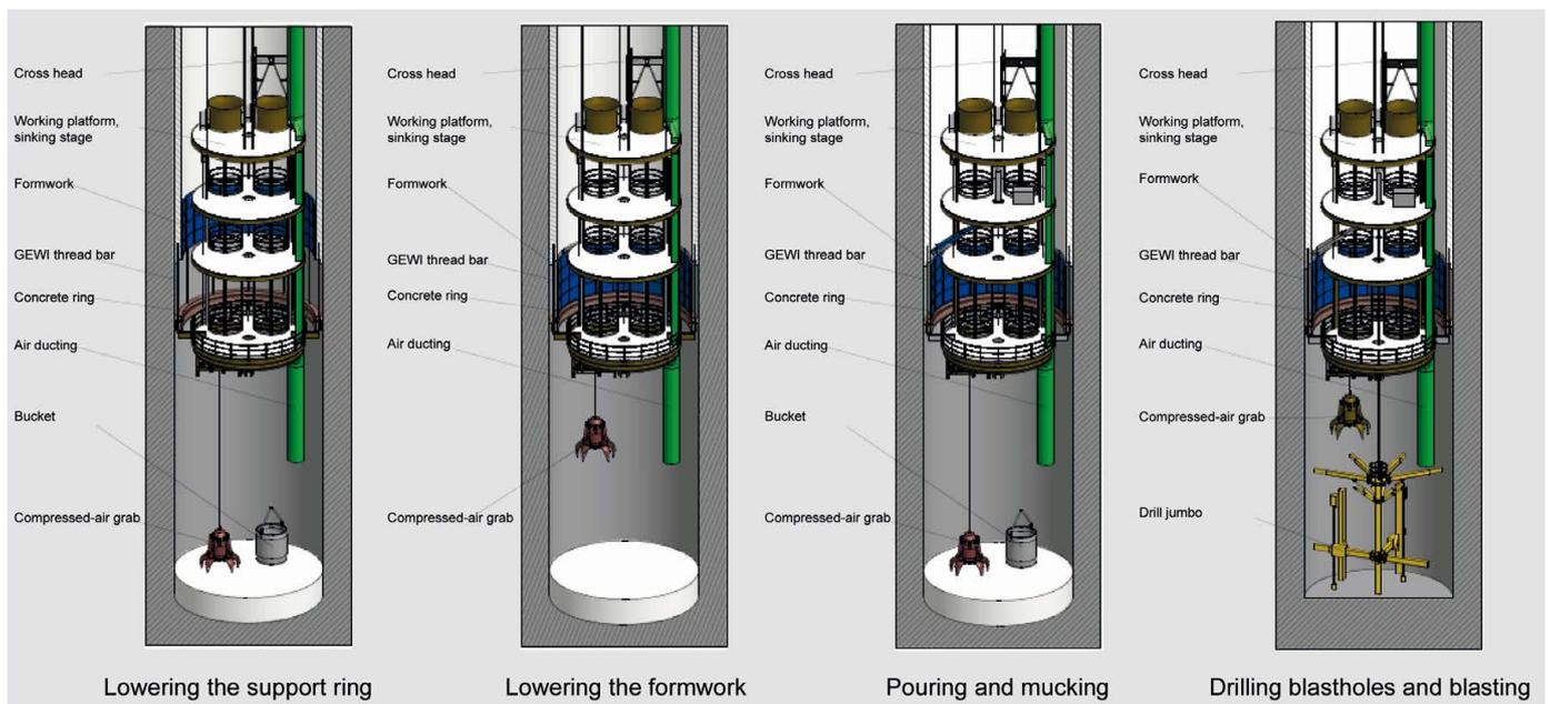
Fig. 7: Key phases in the working cycle of a new shaft excavation
