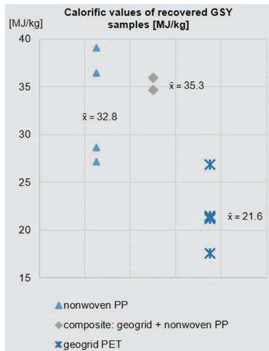
Fig. 9: Calorific values of recovered GSY samples [MJ/kg]
