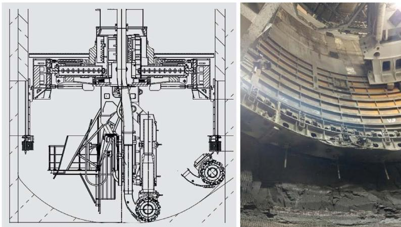
**Fig. 23:** The formwork is reduced in height and brought closer to the shaft floor in order to minimise the risk of further collapses.
