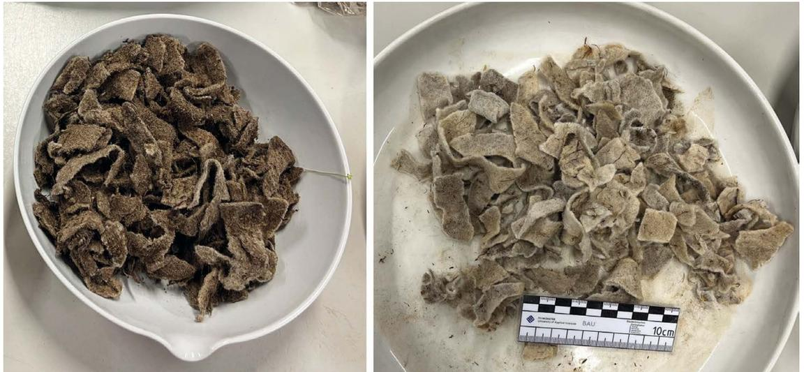
**Fig. 10:** Nonwoven fabric sample before and after partial removal of adhering soil
