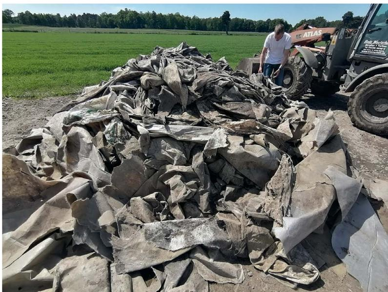
**Fig. 3:** Irregularly torn and soiled nonwoven fabric haphazardly arranged after deconstruction
