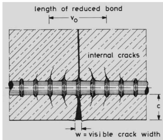
**Fig. 4:** Microcracks forming at every thread crest in reinforced concrete elements; only some cracks extend to the outer edge of the concrete [12]
