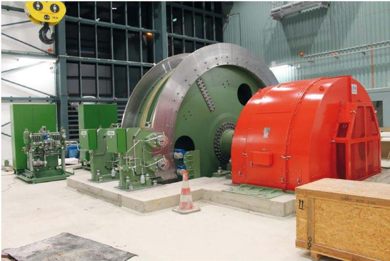
**Fig. 5:** North shaft winder with drive
