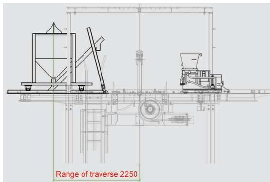
**Fig. 16:** Big Bag unloading process – parked position during the bucket transfer phase
