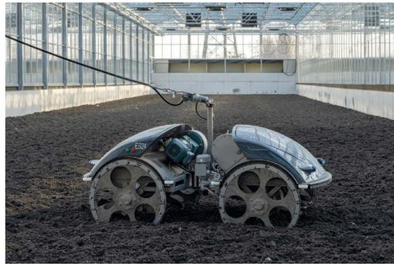
**Fig. 7:** 'Electric hog' in operation at a water treatment works
