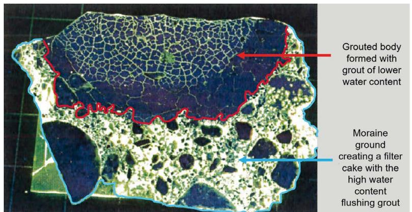
**Fig. 5:** Sample impregnated with an epoxy and viewed under UV Light
