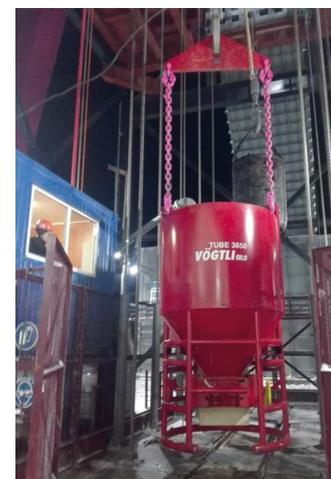
Fig. 19: Concrete bucket with electrohydraulic operation by remote control
