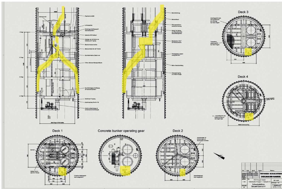
**Fig. 10: A hose line on the shaft scaffold transfers the concrete from the slick line to a secondary mixer on deck 2.**
