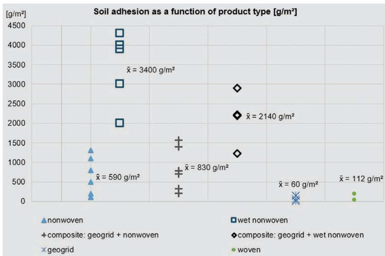
**Fig. 6:** Soil adhesion as a function of product type [g/m²]
