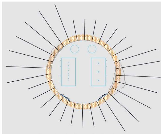
**Fig. 13: Shaft cross-section with shotcrete shell and injection bolts of different length**
