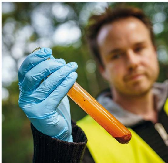
**Fig. 2:** Strongly iron-contaminated mine water from the Dickenberg drift that is used to drain the now-abandoned western working panels of Ibbenbüren colliery. The precipitates are clearly visible as sedimented sludge in the bottom of the test tube.
