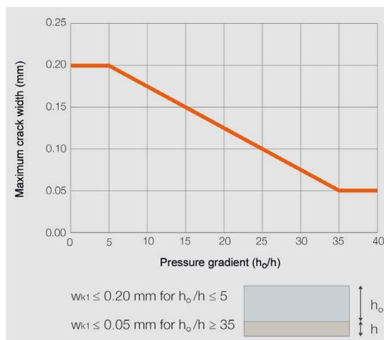
**Fig. 1:** Admissible crack widths for impermeability class 1 and self healing of cracks according to EN 1992-3 [1]
