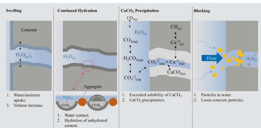
**Fig. 3:** Causes of self healing in separating cracks [4]
