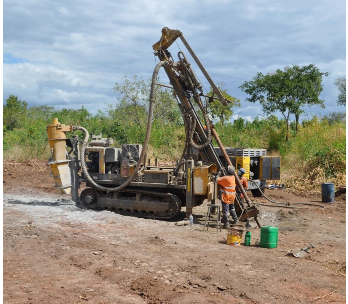
Figure 19: Inclined drill rig as per drill plan
